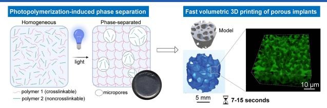
Left: New water-soluble, biocompatible photopolymer resins rapidly form microporous hydrogels via photopolymerizationinduced phase separation. Right: 3D-printed bone-like construct with hierachical porosity by volumetric printing in seconds.
